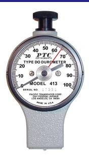
ASTM Type DO measures the indentation hardness of Fireproof Coating, Paint, Moderately Hard Rubber, Elastomers and Dense Textile Windings.
